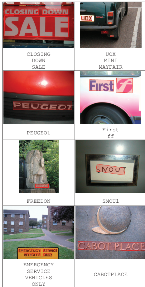
Figure 13: Text localization and recognition examples from the ICDAR 2013 dataset.
