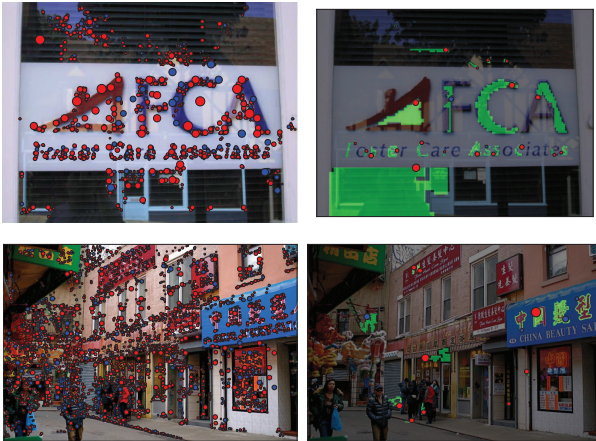
Figure 2: Detected FASText keypoints are effectively exploited to produce stroke segmentations. Detected FASText keypoints (left) and the resulting region segmentations produced by several keypoints selected for illustration purposes (right).
