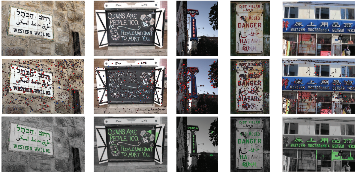
Figure 11: Scene text images with different scripts, fonts and orientations. Source images (top row), detected FASText keypoints (middle row) and resulting text segmentation (bottom row). Best viewed zoomed in color.
