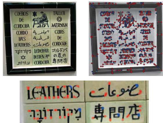
Figure 1: The FASText detector output. Stroke End Keypoints (SEK) marked red, Stroke Bend Keypoints (SBK) marked blue.
